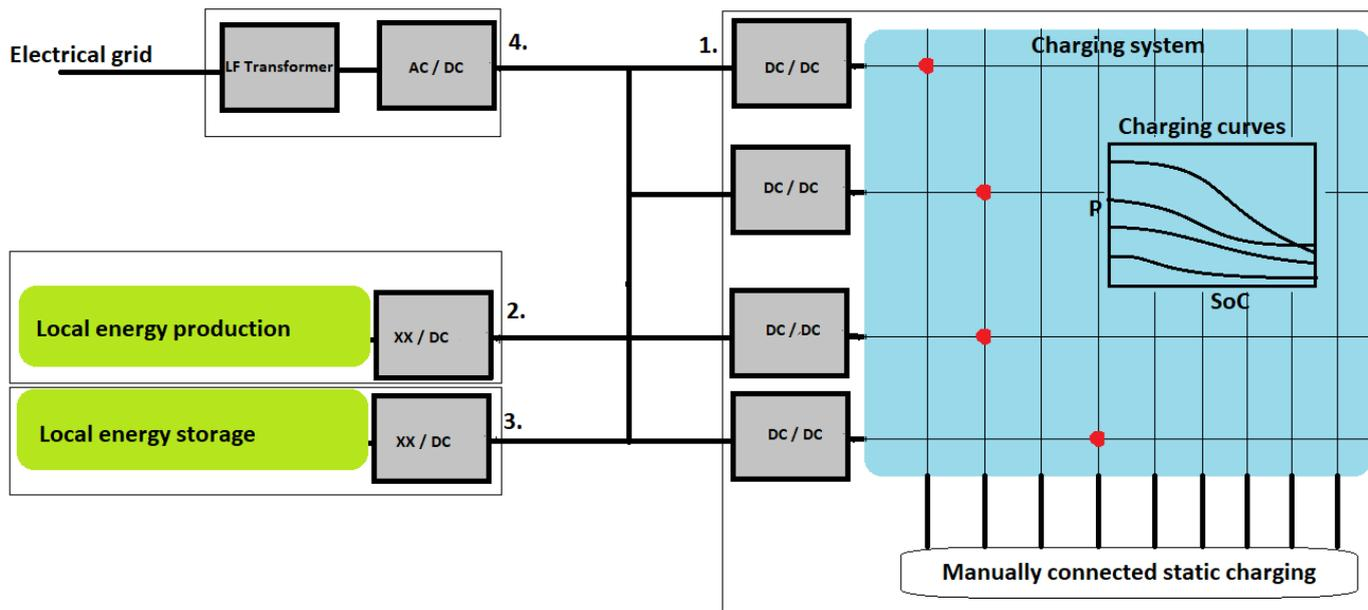
Figure 1: Possible layout of an energy node
