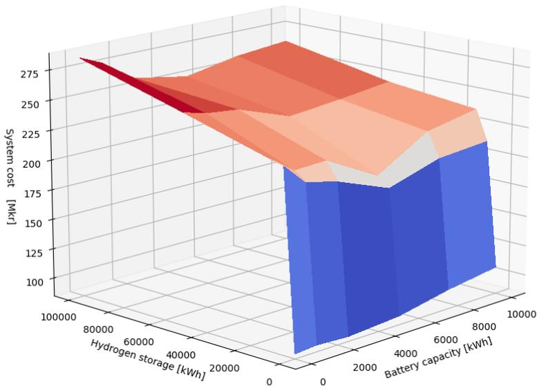
**Figure 31:** System cost of storage combinations in Ekeröd with ten hectare solar panels
