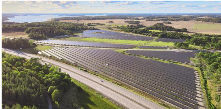
**Figure 14:** Sweden's largest solar farm as of 2022, 35 hectare and 14 MW [36]
