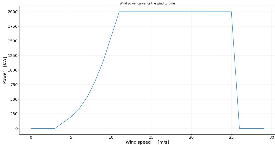
**Figure 15:** Power curve for the chosen wind turbine
