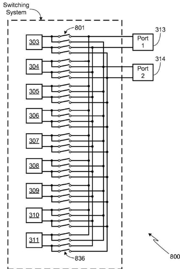
**Figure 2:** Switch system for charging blocks 303-311 from two ports 1 and 2
